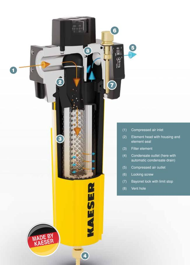
Image: Functional diagram, coalescence filter
