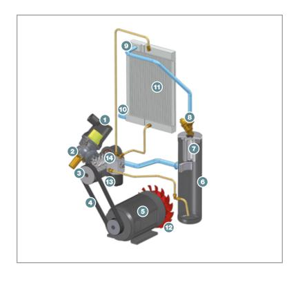
Inlet valve (2) Airend (3) (4) Belt drive (5) IE3 drive motor (6) Fluid separator tank (7) Fluid separator cartridge (8) Minimum pressure check valve (9) Compressed air aftercooler (10)Compressed air connection (11) Fluid cooler (12) Fan Fluid filter (13)
