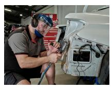
Caption: Compressed air is an essential utility at Charlie Battisti. It is used extensively, from powering the air tools - such as the sanders and polishers - to providing air to the dedicated paint refinish facility.
