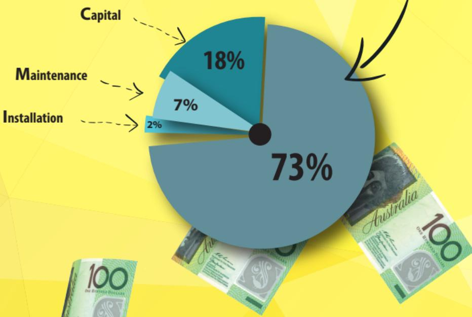
The **lifetime electricity cost** of just one 250 kW compressor, running 3 shifts, 7 days a week with electricity costs at \$0.10/kWh will therefore equate to
