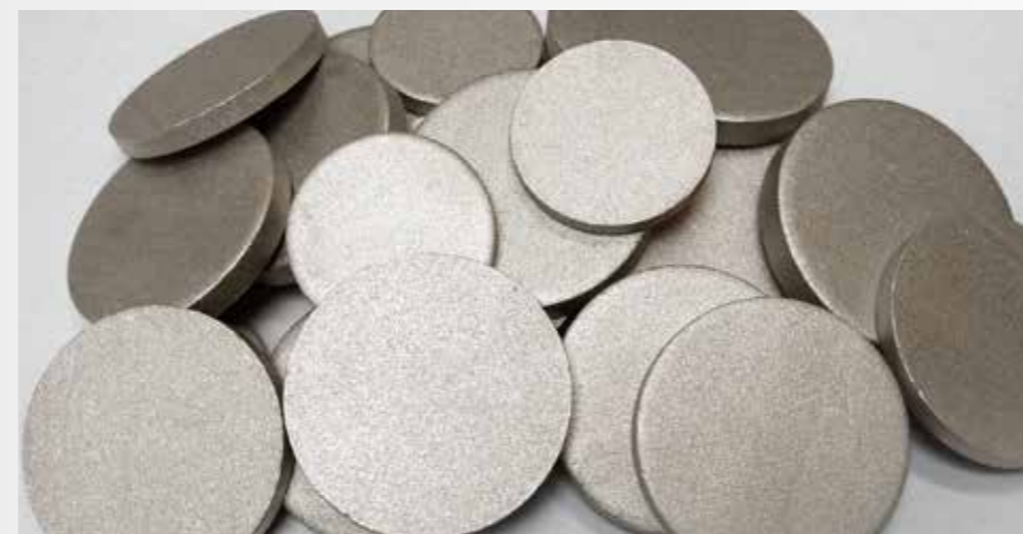
The raw material for the aerosol cans resembles metal coins.
