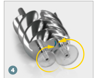
4 Flow chamber completely evacuated
